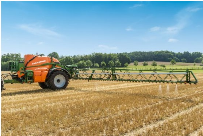
A 24m (78ft) version of the Amazone UX trailed sprayer is the first to be offered with the AmaSpot weed-detecting and spraying system.
